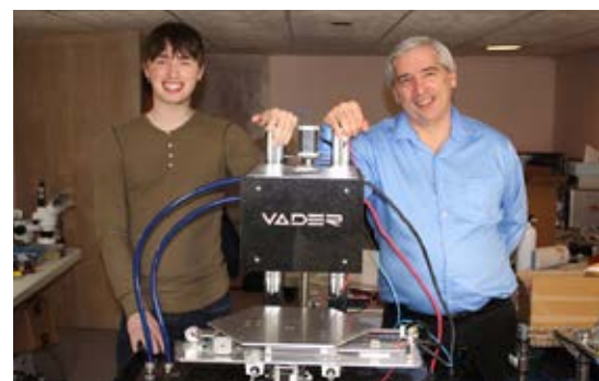
From left, father-son team Zachary and Scott Vader pose in their basement with their invention, a 3D printer that uses liquid metal jet printing.
