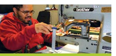
Ted Zrimsek works on a modified, hand-operated bar tacker at TRC's Work Center in Dunkirk. A hand lever was added to Ted's sewing machine because he cannot operate a foot pedal.
