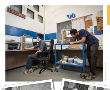
LEFT: Xinnan Peng and Courtney Scott utilize new digital CNC simulators, which replaced the analog instrumentation used to control the milling machines.
