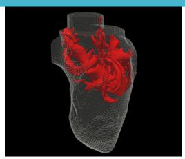
MAE researchers are using computational fluid dynamics (CFD) to improve the design and placement of cardiovascular devices such as artificial heart valves.
