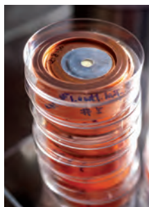
Stack of membranes, each housed at the center of a copper and aluminum disc that helps to protect the material during experiments.
