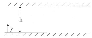
At time t = 0 the velocity V(y,0) = 0. At time  $t = 0^+$  both plates are suddenly accelerated to and then maintained at a velocity  $V(h,t) = V(0,t) = V_0$ .
