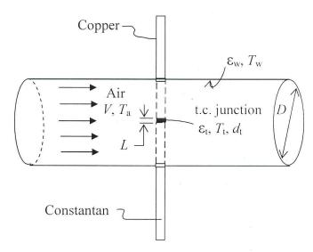
A thermocouple (t.c.) junction of diameter  $d_t$  and length L has been designed as shown above. Its purpose is to measure the temperature of the air flowing through the duct. Calibrations, however, always indicate a difference between the air and the thermocouple temperatures. The objective of this analysis is to determine the reason for this 'thermocouple error' and calculate its value:  $(T_t - T_a)$ .
