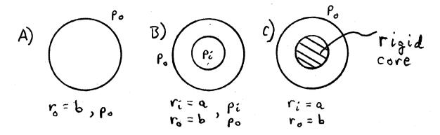
b) If there is a single cylinder of format "B" with inner pressure equal to zero and there are no end caps, consider the shape of the curves for the stresses  $\sigma_r$  and  $\sigma_\theta$ .
